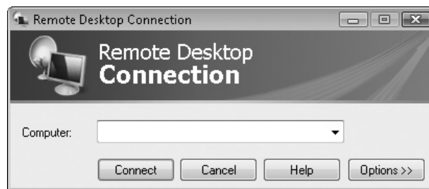
FIGURE 8-7 The Remote Desktop Connection tool is used to connect to the server.
