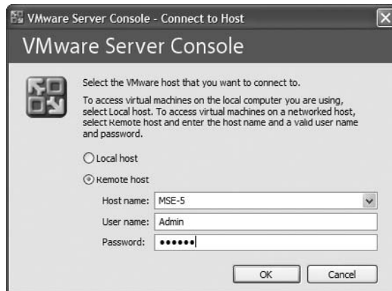
FIGURE 13-5 The VMware Server Console allows you to connect to your virtual servers.
