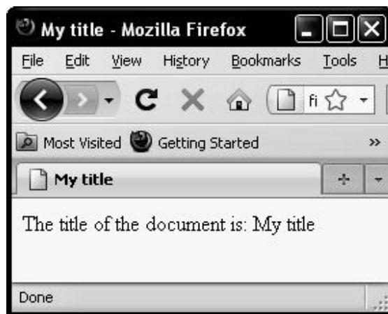
Fig 8.3 Script and output Demonstrating write method and title property of Document object.
